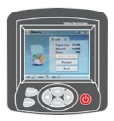
Press "SNAP" and "RECORD" to select the current memory medium (SD/Flash), select "Work space" and press "OK" button to confirm.
