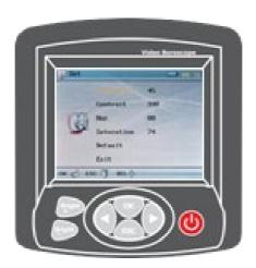
Press "SNAP" and "RECORD" button to increase or decrease the value to adjust the effect of the camera. (The adjustment will produce a slight effect and only can be identified in the camera mode.
