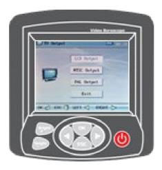
Select the "NTSC" or "PAL" respectively in accordance with the video format of television, and press "OK" button to enter. The content will still be controlled with the instrument but
