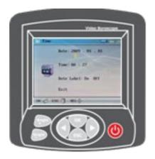
Move the cursor with the Right/Left button to the functions you want to set up, then press "SNAP" and "RECORD" to adjust the date and time.
